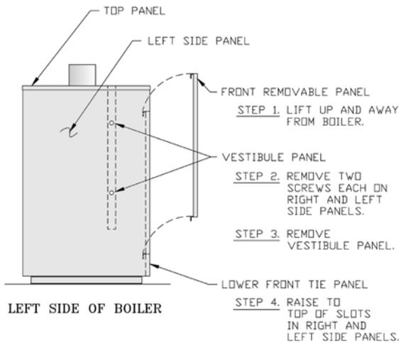
**Figure 18: Jacket Front Panel and Vestibule Panel Removal**
