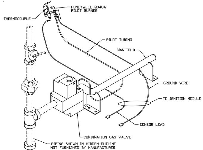
**Figure 7: Pilot and Gas Piping, Intermittent Ignition (EI)**
